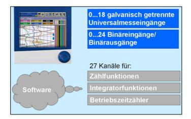
These are **not** electrical measurement inputs (hardware), but channels which are calculated by the paperless recorder (software).
